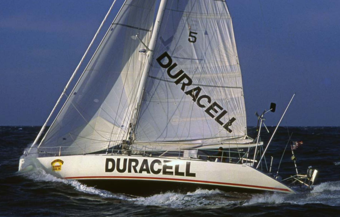
Duracell storming along with a reef in her main and her smaller jib set. Mike's onboard power was augmented by the wind generator seen just aft of the boom. The wind vane self-steering unit is visible on the stern. (Billy Black)
