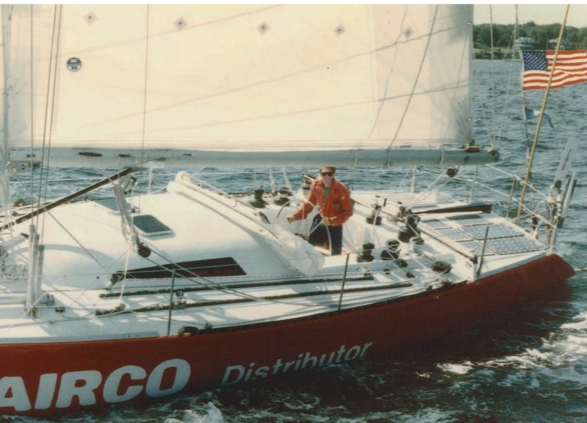
Mike at the wheel of Airco, Newport, Rhode Island. Note the wind vane self-steering unit hung off the stern—some system of self-steering is vital for singlehanders. (Billy Black)
