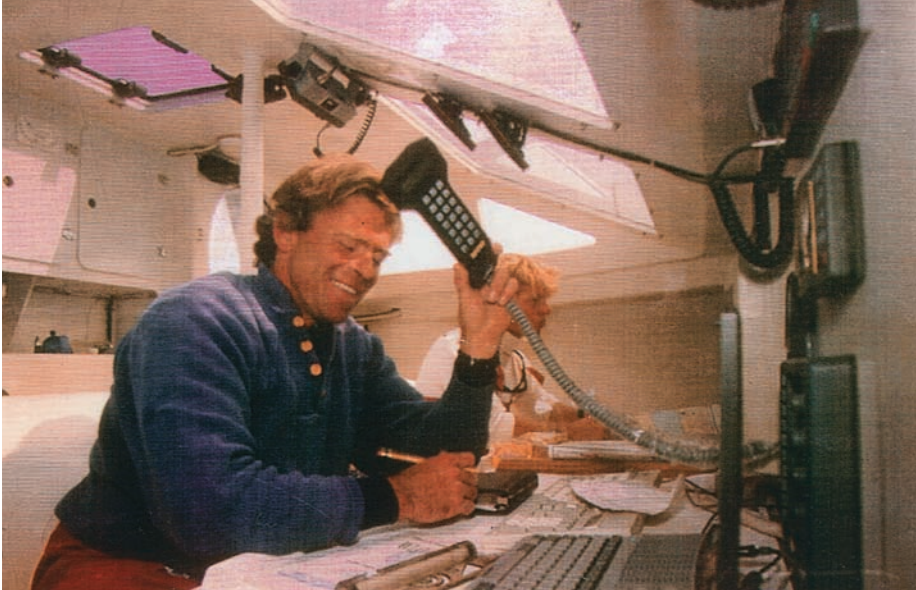
Mike at the navigation station on Duracell. Ocean racers kept in touch with shoreside crew and other competitors and obtained important navigational information via multiple electronics, such as VHF, SSB radio, and weather faxes. Other onboard systems also relied heavily on power: early GPS units, autopilots, radars, bilge pumps, and pumps to move water ballast between tanks. (Billy Black)
