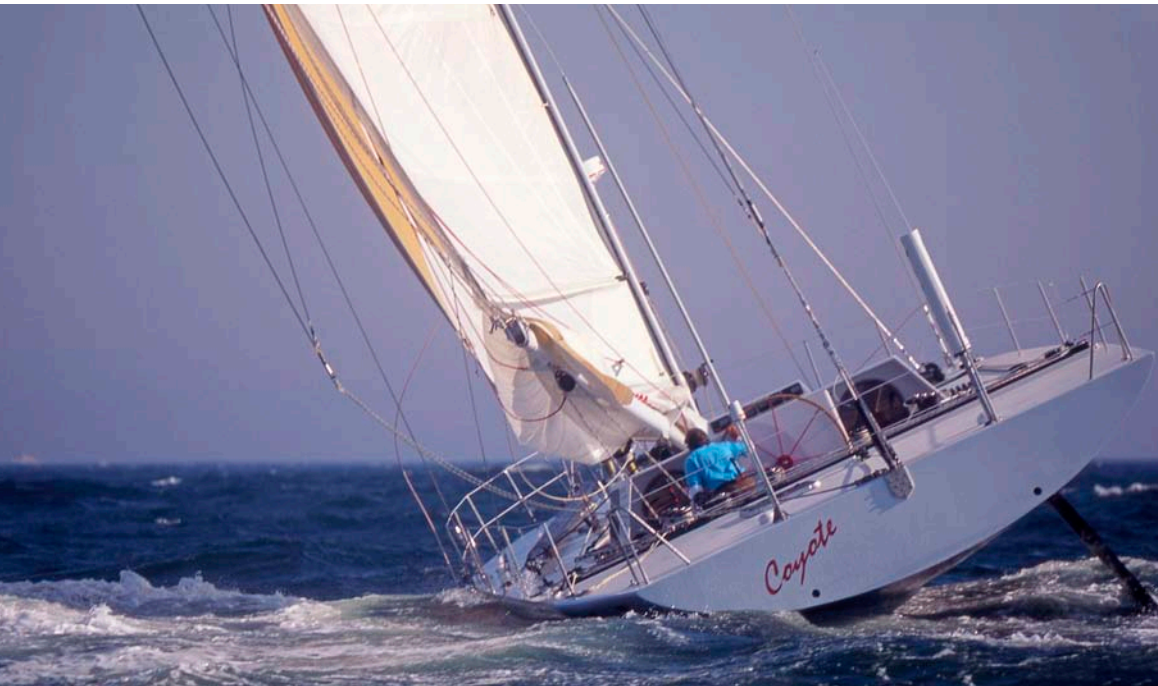
Top: Mike on Coyote's foredeck. Below: Coyote with a reef in her main, from the stern. Her wide beam is readily seen in this view. Water ballast tanks allowed Mike to adjust Coyote's angle of heel. (Billy Black)
